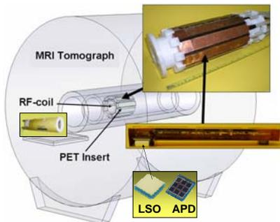
Figure 1: Developed PET/MRI System of Tübingen. The PET insert is composed of ten block detectors using a 12x12 LSO matrix which is read out with a 3x3 APD array. APD-PET signals are lead outside the 5 Gauss fringe line and processed to listmode data.
